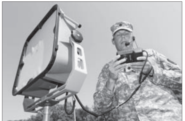
In this photo taken Sept. 14, 2011, Lt. Col. Jeffrey Bevington, requirements officer with the Joint Non-Lethal Weapons Directorate, demonstrates one of the military's latest voice projection system and instant translation technologies, that can project a human voice a mile away and instantly translate from English to another language, at the Marine Base in Quantico Va. Associated Press
